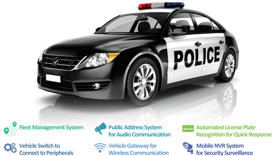
Figure 4 In a police car, a vehicle server can handle ALPR, mobile NVR, public addressing, vehicle switch and gateway, and fleet management at the same time.
